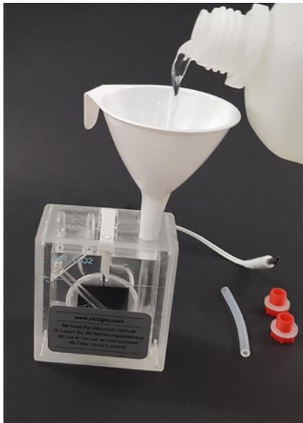
Pour sodium chlorite up to the mark carefully.
