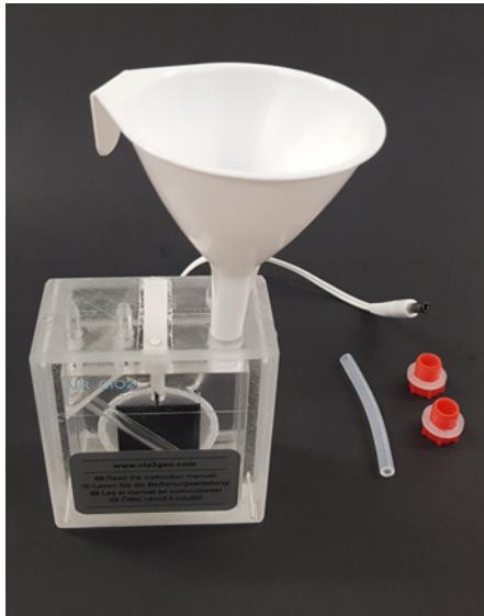
Carefully attach the funnel to the generator drain.
