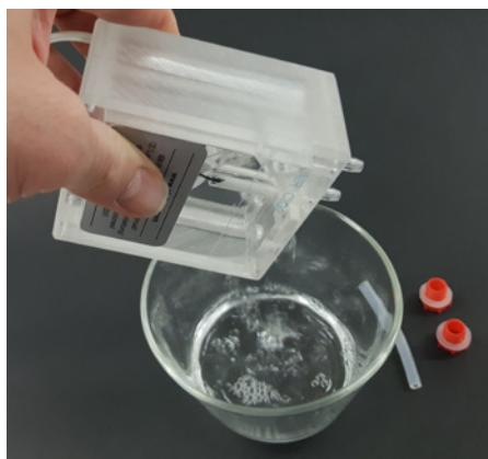
*Drain the water inside the generator into a container. Then pour the water from the container into the drain.*
